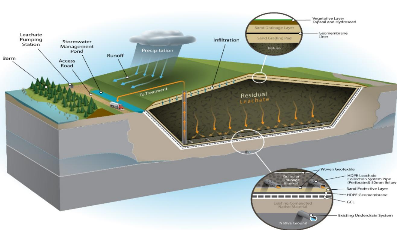
will make it safer by improving the cell liners and leachate collection system. At the end of the cleanup, leachate will be directed to a buried tank, which will be regularly pumped out and disposed of at an off-site wastewater treatment plant. The top of the containment cell will be capped, and long-term monitoring will continue after the cleanup to ensure the cell is working as planned.
